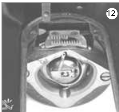
(11) Remove the cover plate by lifting the outside edge very slightly and twisting the plate with a little pressure towards you and upwards.
