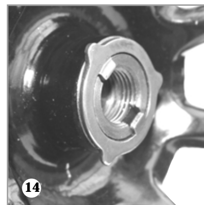
(14) Now the clamp stop motion (or clutch) washer has been added and you can see how the two inside lugs fit into the two notches at the end of the shaft.
