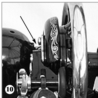
(10) Check if the bobbin winder attaches at the top of the machine.
