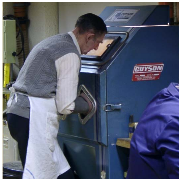
Above: volunteer Syd uses the shot-blasting cabinet to clean a badly rusted tool.
